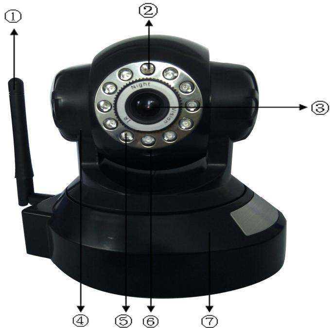
①---WIFI antenna; ②---LDR(light dependent resistor); ③---lens; ④—PTZ; ⑤——Infrared lamp; ⑥---Microphone; ⑦---Base;
