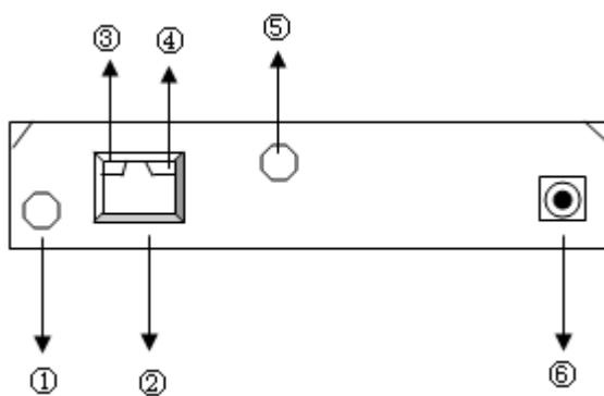
①---Audio output; ②---Network port; ③---web working station indicator; ④—Power light;
